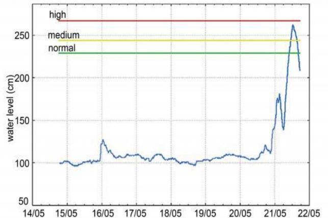
WATER LEVEL CHART TRACKING OF LAMBRO RIVER SOURCED FROM METEOROLOGICAL DATA, 21/02/2012 FROM THE CHART ABOVE, WE CAN SPECULATE THAT WATER LEVEL OF THE RIVER FLUCTUATES AROUND 1.8 - 2 METERS IN THE RAINY SEASON
